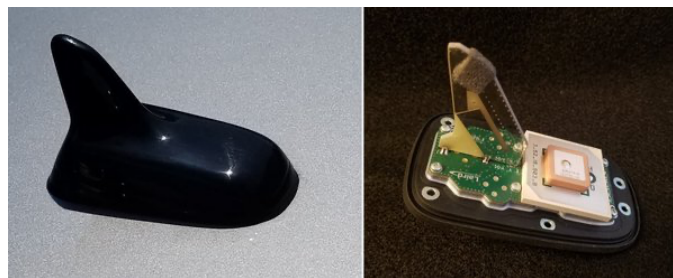
FIGURE 18: SHARK FIN ANTENNA SYSTEM
