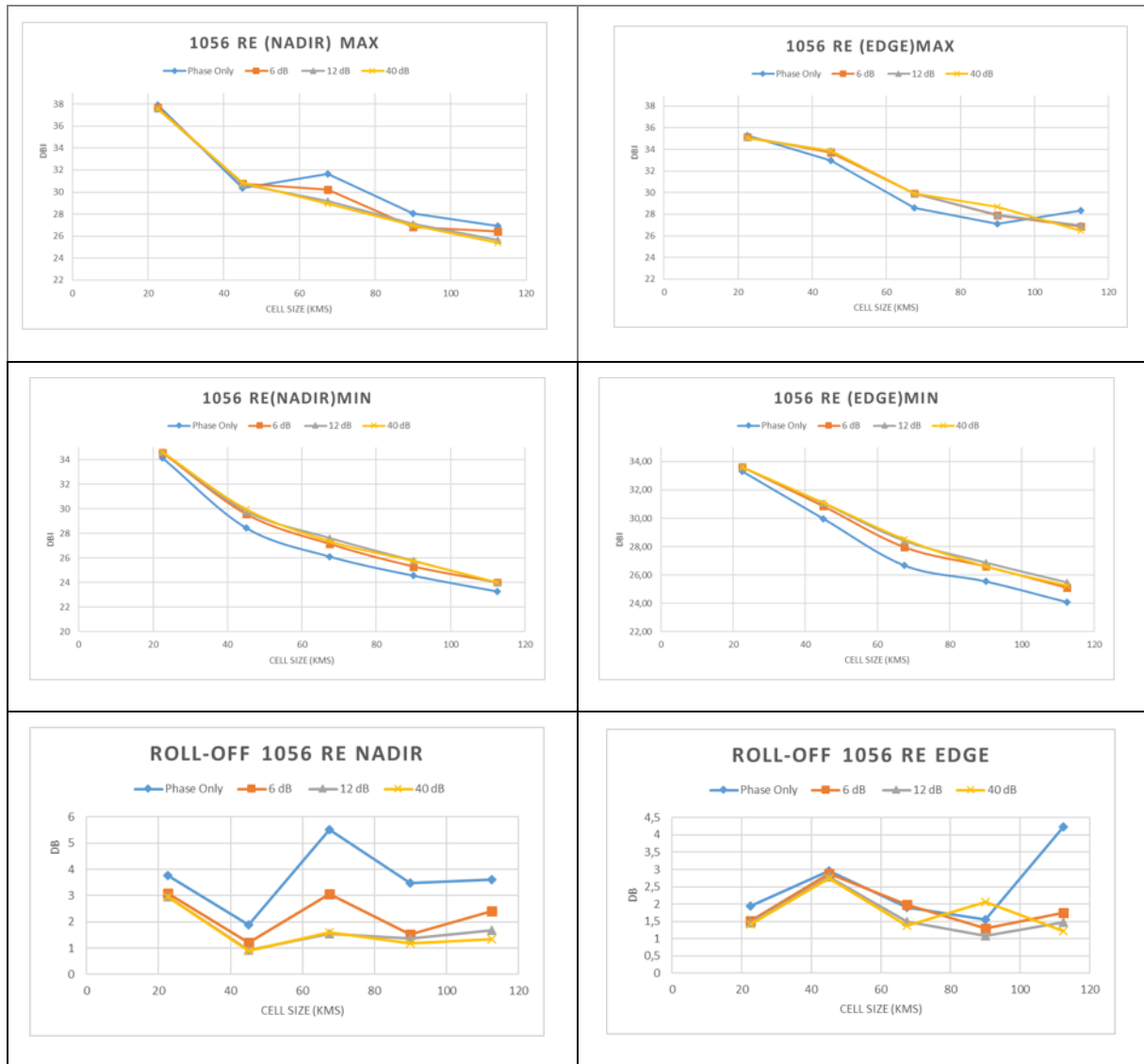
FIGURE 4-31 ANTENNE 1056 RE 0.741λ : directivity min and max over cell at nadir and edge
