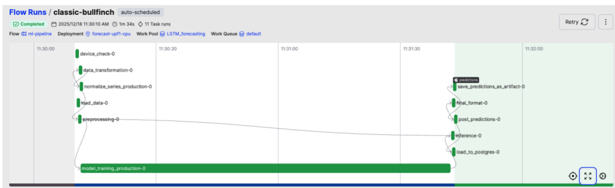
FIGURE 6: ML FORECASTING PIPELINE ORCHESTRATED AS A PREFECT FLOW
